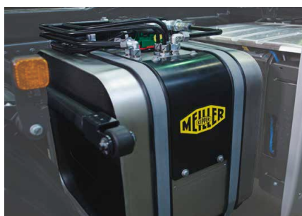
Everything from a single tank: Several consumers (tipper, crane & hydraulic system for municipal services) can be supplied from one compact MEILLER tank.
