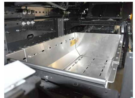
Room used optimally: toolbox between the axles.
