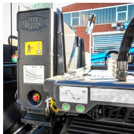
MEILLER control unit with integrated overload control display (standard with telescope equipment)
