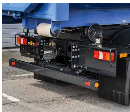
Rear underrun protection always in the correct position: slides in when tipping and rolling off, extended when driving.
