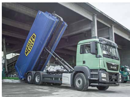
More room to manoeuvre under roofed areas due to the lower superstructure of the hooklift.
